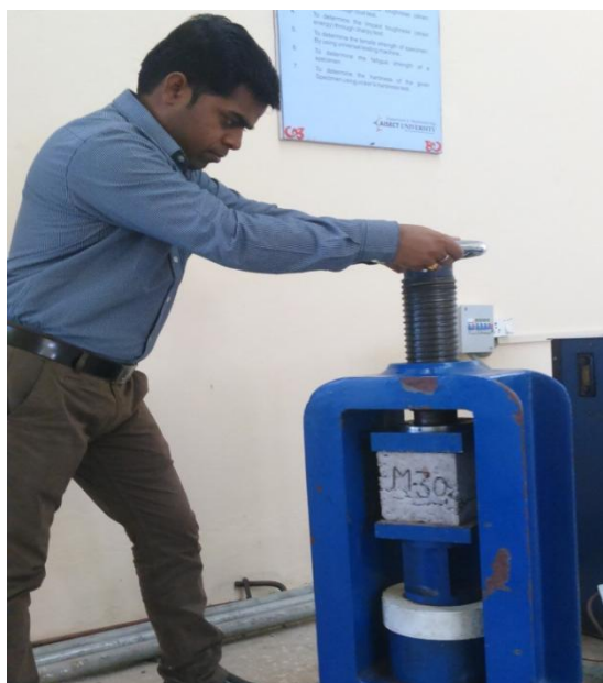
Fig.3: Compressive strength test of cube specimen on Compression testing machine.
