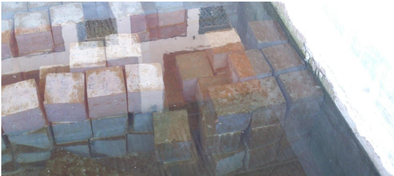
Fig.2: Wet curing of specimens
