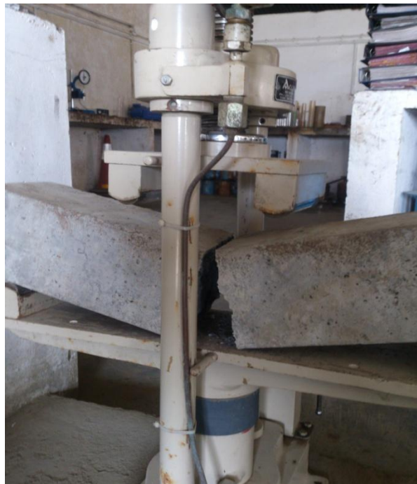
Fig.4: Flexural strength test of Beam specimen on third point loading apparatus.
